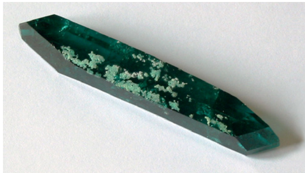
Figure 13. Malossi hydrothermal synthetic emeralds have been available in the trade since 2004. The rough specimen on the left (~6 cm long) is partially encrusted with white synthetic phenakite crystallites. Photos by Ilaria Adamo.
