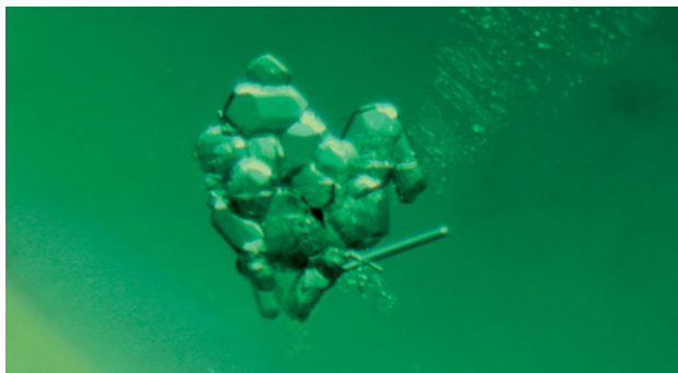
Figure 14. A cluster of small inclusions, probably synthetic phenakite, were observed in this Malossi hydrothermal synthetic emerald. Photomicrograph by Renata Marcon; magnified 50 \times .
