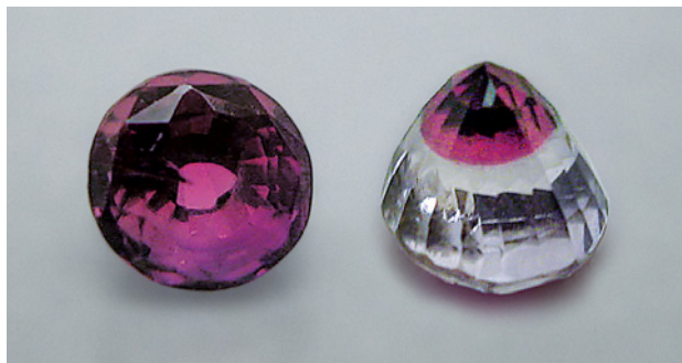
Figure 7. To produce a novelty, flame-fusion synthetic rubies and sapphires can be easily cut from areas within a boule where near-colorless portions join with the colored overgrowths. When this is done, a strongly color-zoned synthetic is the result, as shown by this 1.05 ct example. Composite photo by H. A. Hänni, © SSEF.
